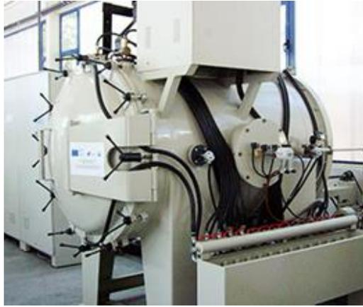
**Fig. 8** – *Vacuum furnace for thermal and chemical-thermal treatment of metals with pulse glow discharge.*
