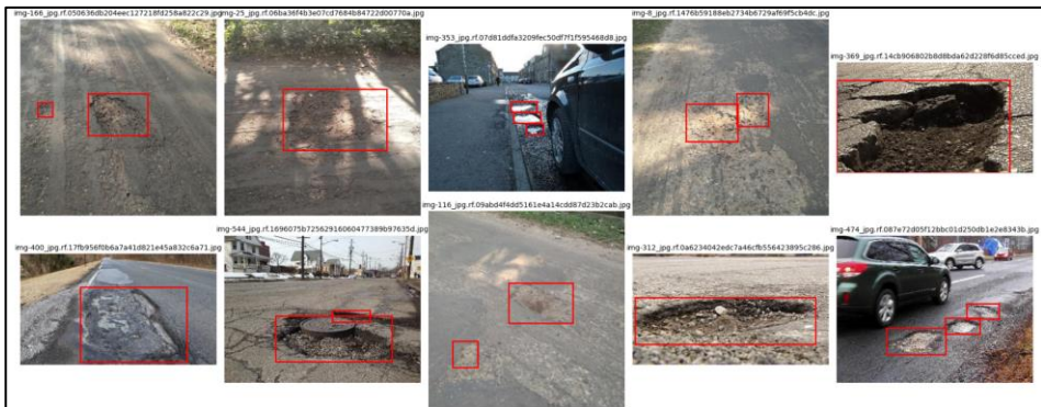
Fig. 3 – Camera-captured road scene with EfficientDet-based pothole detection.
