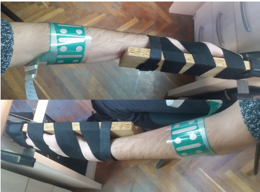
Fig. 1 – Hand immobilization of healthy able bodied subjects. The novel flexible electrode for recording EMG signals is wrapped around the subject forearm.
