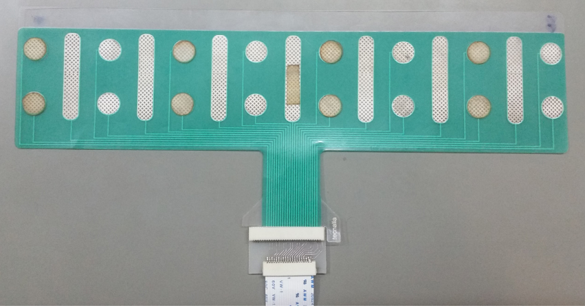
Fig. 2 – Flexible matrix electrode for recording EMG designed by Tecnalía Research & Innovation, San Sebastian, Spain.
