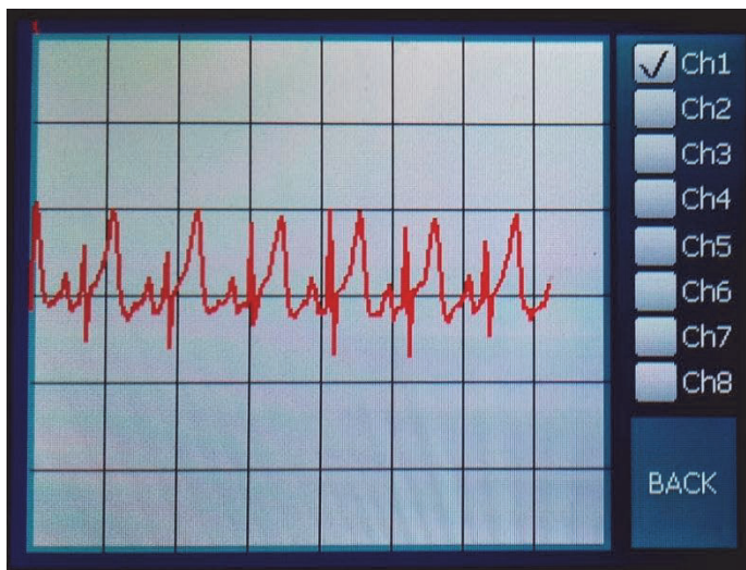
Fig. 8 – ECG signal displayed in duration of 5s with maximal display amplitude range of 1 mVpp.
