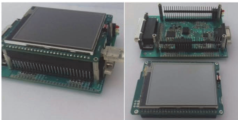
Fig. 2 – The physiological data acquisition system, assembled (on the left) and unfolded (on the right).
