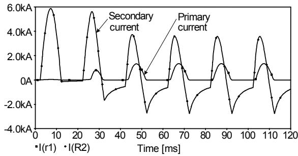
**Fig. 8 – Primary and secondary current – heavy saturation.**
