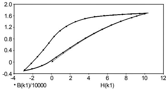
**Fig. 7 – Switching transients simulation of  $B(H)$  loop –  $\beta = \pi/4$ .**
