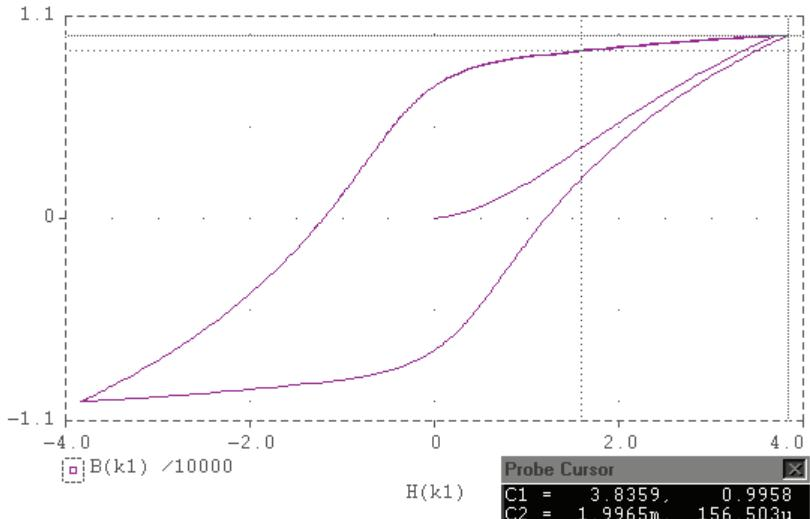
**Fig. 1 – Simulation of  $B(H)$ .**
