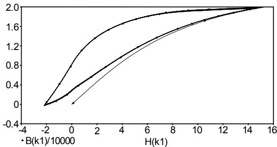
**Fig. 5 – Switching transients simulation of  $B(H)$  loop -  $\beta = 0$  .**
