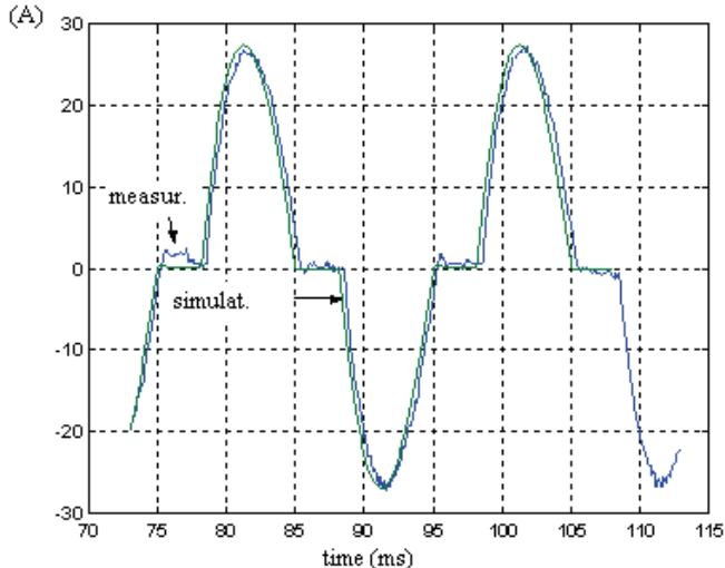
**Fig. 3 – Measured and simulated current in the case of phase control.**
