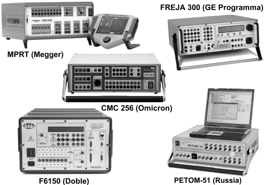
Fig. 3 – The modern computerized test systems of last generation for testing of multipurpose microprocessor based protective relays.
