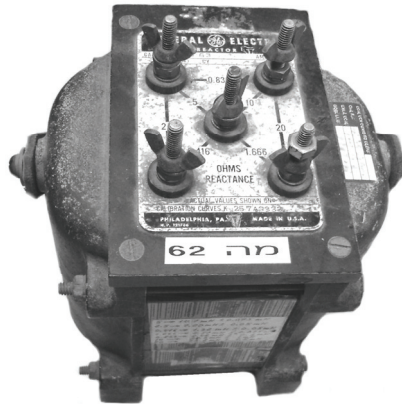
Fig. 1 – Set of inductances from General Electric for testing of electromechanical protective relays.
