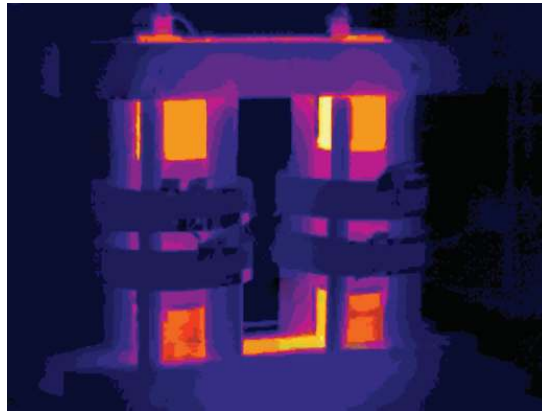
Fig. 8 – The temperature distribution in ferrite core.
