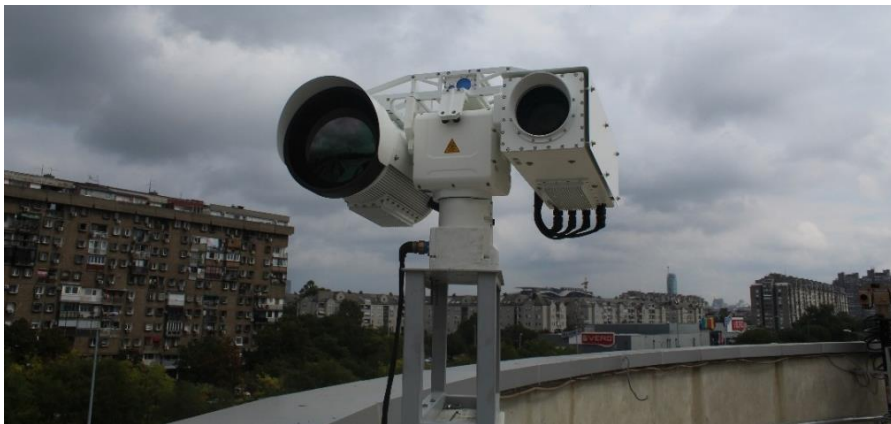
Fig. 1 – Experimental setup of the multi-sensor EO/IR platform during the stationary field measurements.
