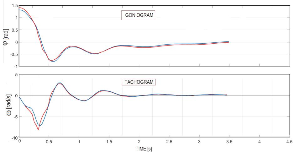
**Fig. 9 –** Knee joint goniogram and tachogram for Subject 2 (patient) estimated by image analysis of the movie recorded (red line) and the signals from the joint angle encoder (blue) for the pendulum test.
