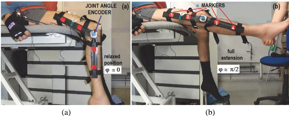
**Fig. 1 – (a)** The neutral position of the leg showing the joint angle encoder as described in Popović Maneski et al. [5]. **(b)** The fully extended leg with passive markers. Four red squared markers along the thigh (1 and 2) and shank (3 and 4) determine the directions of the upper and lower leg.
