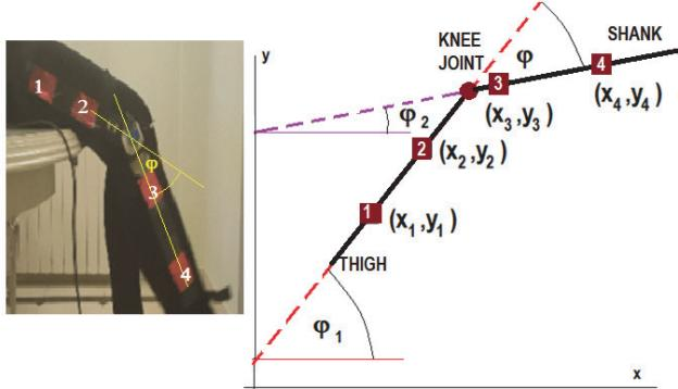
**Fig. 2 – Sketch of the markers (1, 2, 3, and 4) and angles used for the calculation of the knee joint angle  $\varphi$ . Coordinates  $(x_1, y_1)$  and  $(x_2, y_2)$  define the thigh direction  $\varphi_1$  vs. the horizontal line. Coordinates  $(x_3, y_3)$  and  $(x_4, y_4)$  define the direction of the shank  $\varphi_2$  vs. the horizontal line.**
