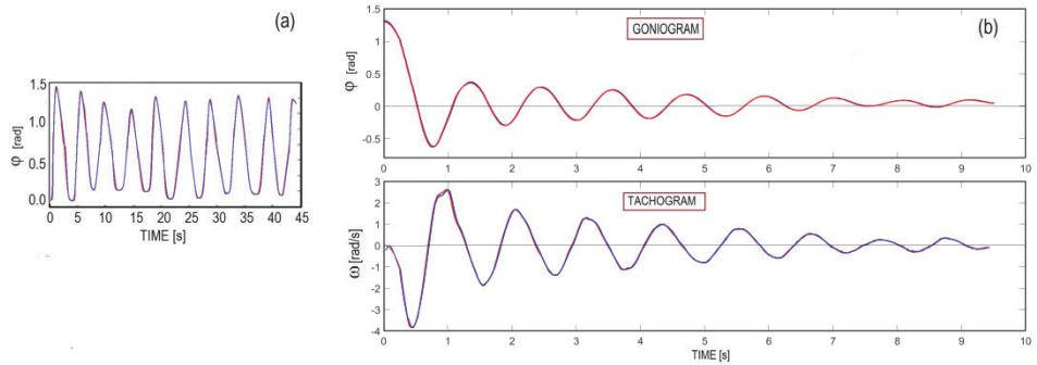
**Fig. 8 –** (a) Superimposed angles estimated from the camera data (red line) and the data from the angle encoder (blue line) for ten consecutive voluntary movements of the lower leg from the flexed position to the near full extension and back (Subject 1).
