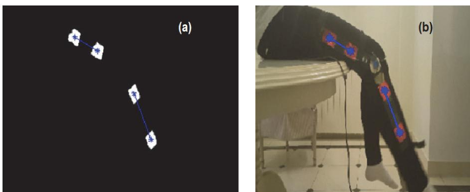
**Fig. 7** – (a) The image after morphological operations and detection of centroids.
