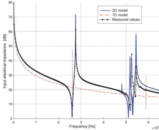
**Fig. 4 – Simulated and experimental input electrical impedance versus frequency for the Transducer1.**
