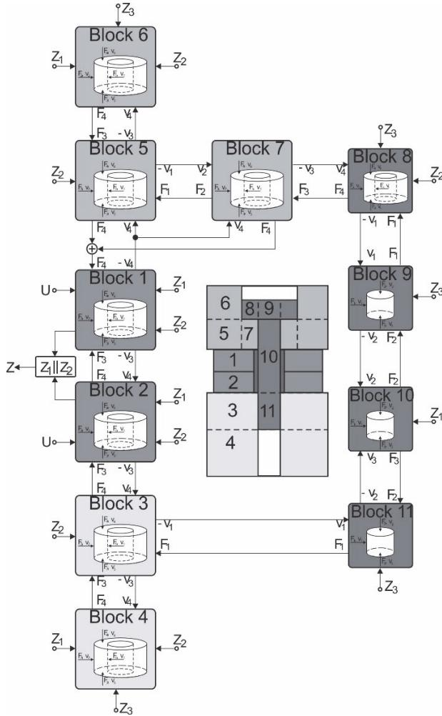
**Fig. 1 – Block diagram of the ultrasonic transducer model.**
