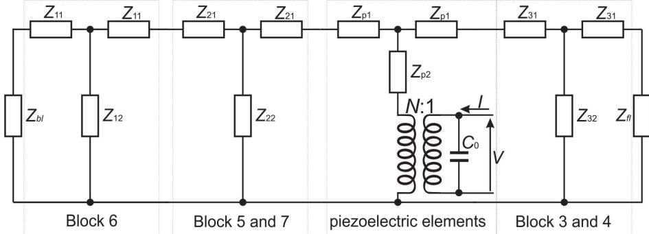
**Fig. 2 – Electromechanical equivalent circuit of the unsymmetrical ultrasonic transducer.**
