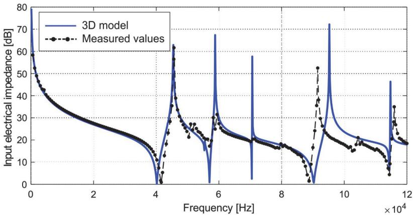
**Fig. 5 – Simulated and experimental input electrical impedance versus frequency for the Transducer2.**
